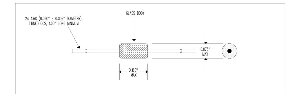
RESISTANCE @  $+25^{\circ}C = 2,000,000 \ \Omega \pm 10\%$  RESISTANCE TEMPERATURE CURVE = "V4" TEMPERATURE COEFFICIENT @  $+25^{\circ}C = -4.85\%$ /°C NOMINAL BETA " $\beta$ " (0 TO  $+50^{\circ}C$ ) =  $4,288^{\circ}K$  NOMINAL (STILL AIR) THERMAL TIME CONSTANT = 2 mW/°C NOMINAL (STILL AIR) THERMAL TIME CONSTANT = 0.5 SECONDS NOMINAL (STIRRED OIL) MAXIMUM TEMPERATURE RATING =  $+300^{\circ}C$
