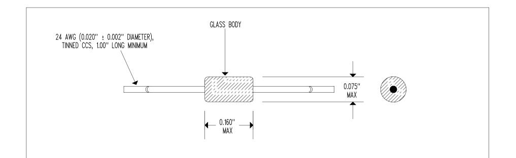
RESISTANCE @  $+25^{\circ}C = 5,000 \ \Omega \pm 10^{\circ}$ RESISTANCE/TEMPERATURE CURVE = "F"
