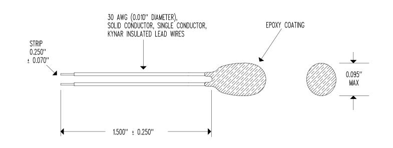
RESISTANCE @  $+25^{\circ}C = 10,000 \Omega$  NOMINAL ACCURACY (0 TO  $+70^{\circ}$ C) = ± 0.20°C RESISTANCE/TEMPERATURE CURVE = "J"
