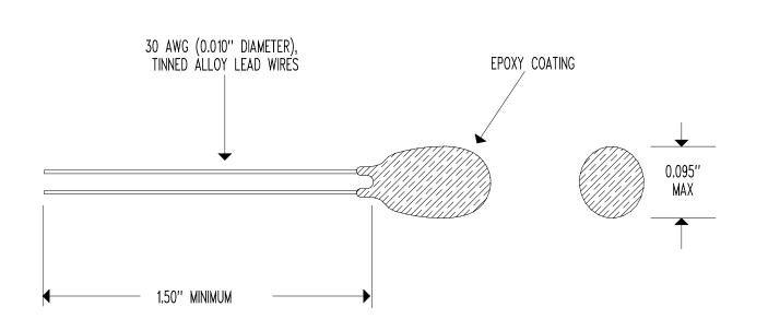
RESISTANCE @  $+25^{\circ}C$  =  $20,000 \Omega$  Nominal accuracy (0 to  $+70^{\circ}C$ ) =  $\pm$  0.20°C resistance/temperature curve = "J" temperature coefficient @  $+25^{\circ}C$  = -4.4%/°C nominal beta " $\beta$ " (0 to  $+50^{\circ}C$ ) =  $3,892^{\circ}K$  nominal dissipation constant = 1 mW/°C nominal thermal time constant = 10 seconds maximum (still air) thermal time constant = 1 second maximum (well stirred oil) maximum temperature rating =  $+150^{\circ}C$
