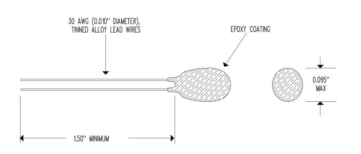
RESISTANCE @  $+25^{\circ}C = 10,000 \Omega$  NOMINAL ACCURACY (0 TO  $+70^{\circ}$ C) = ± 1.0°C RESISTANCE/TEMPERATURE CURVE = "G"
