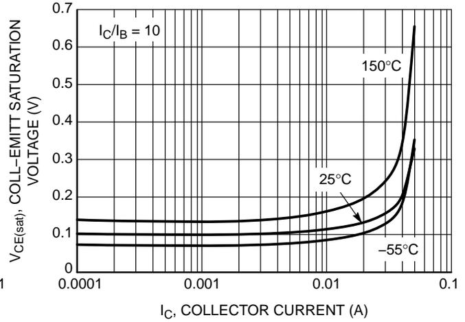
Figure 2.  $V_{CE(sat)}$  Curve
