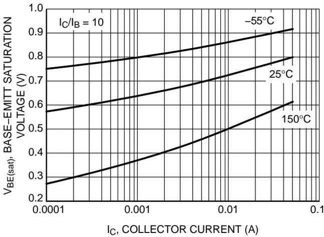
Figure 3.  $V_{BE(sat)}$  Curve
