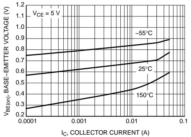
Figure 4.  $V_{BE(on)}$  Curve
