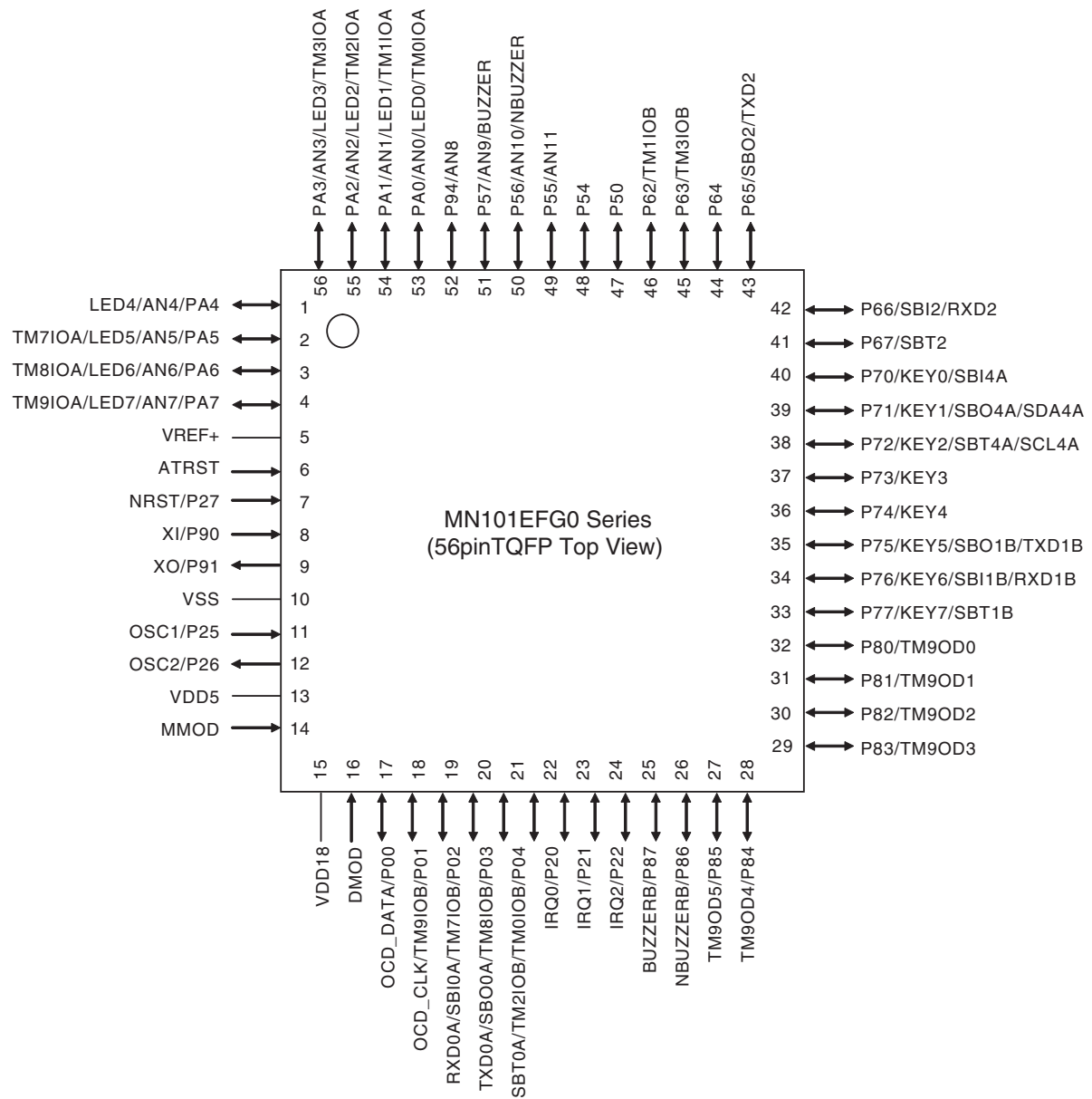
Figure:1.3.5 Pin Configuration (MN101EFG0 Series 56-pin TQFP)
