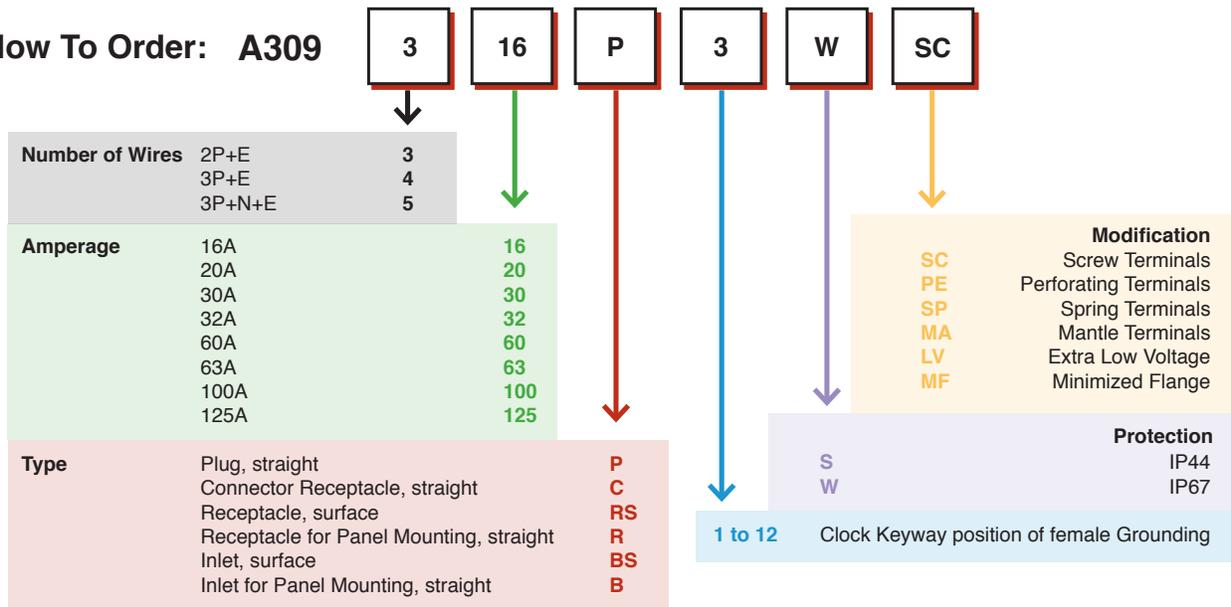
The voltage is determined by the location of the female ground contact relative to the housing keyway. Simply by manufacturing the device with a ground contact in a certain "clock" position, the device will be rated for a particular voltage system.
