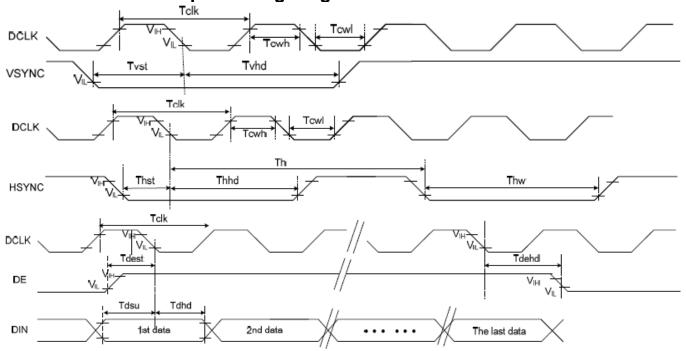
7.2 Serial RGB input timing requirement
