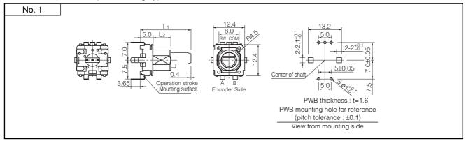
• Standard rotation-torque / Bushing Type with Sleeve / with Switches .......With detents : EVEJBE
