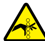
W3153 Pinch Point Hazard
