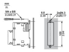
**Digital Transistor Output Module (8-channel, Sink)**
