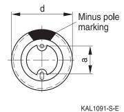
The series B41897 and B41898 have no sleeve nor minus pole marking, the positive pole is marked on the aluminum case side instead.
