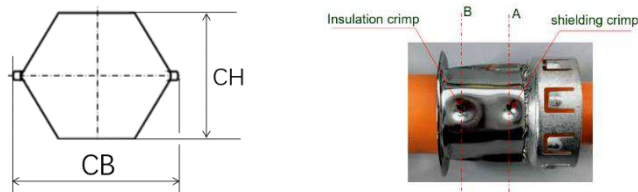
Figure 13: shielding crimp Height and Width
