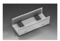
The ERmet shroud type E is possible for a maximum of 220 contacts in 10 rows by 25 positions with the length of 50 mm. The two outer rows, z and y are for the shielding contacts of the female connector. For this type; without multifunction block for coding and pre-alignment, we recommend use only in combination with types D or F.
