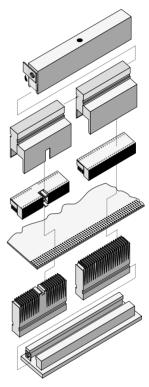
Modular press-fit tool for female connector modules 5+2
