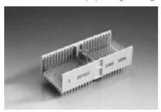
The ERmet type D vertical male connector provides up to 176 signal contacts and 44 ground shield contacts in 8+2 row x 25 position (3 positions used by multifunction cavity), fully loaded configuration. With 15 different standard pin lengths to choose from, this is one of the most versatile connectors available. The connector is designed for gas tight pressfit installation.
