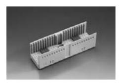
The ERmet shroud type A is possible for a maximum of 175 contacts in 7 rows by 25 positions. The two outer rows, z and f are for the shielding contacts of the female connector. This type contains a multifunction block for coding and prealignment which uses 3 positions.
