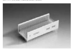
The ERmet type E vertical male connector provides 200 signal contacts and 50 ground shield contacts in an 8+2 row x 25 position fully loaded configuration. This connector is also available in an 8+2 row x 22 positions and 8+2 row x 19 positions. With 15 different standard pin lengths to choose from, this is one of the most versatile connectors available. The connector is designed for gas tight pressfit installation.
