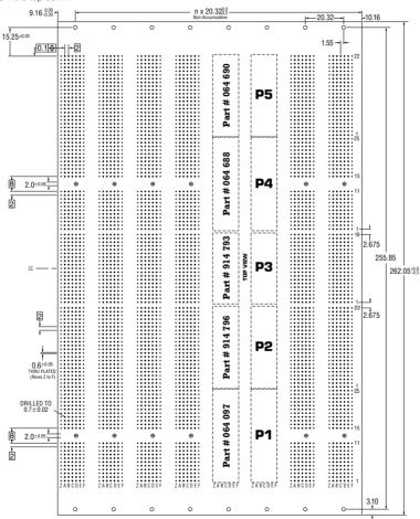
Note that the backplane is numbered in accordance with the CompactPCI® specification. The numbering on the connectors themselves is different and in accordance with the IEC 61076-4-101 standard. All dimensions are in millimeters (mm) unless otherwise noted.
