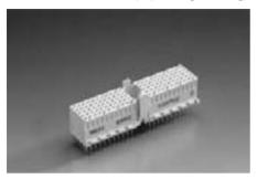
The ERmet type A vertical female connector provides 110 contacts in a 5 row x 22 position fully loaded configuration. Versions with optional "z" and "f" row shields are available as well as extended terminals for use in stacking applications with rear shrouds.
