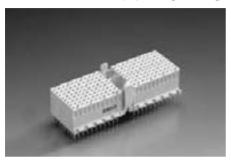
The ERmet type D vertical female connector provides 176 signal contacts in a 8 row x 25 position (3 positions used by multifunction cavity), fully loaded configuration.
