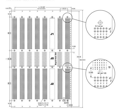
Note that the numbering of the P0 connector conforms to IEEE 1101.1 and 1101.10 and is from the top down. This also is the same numbering scheme established by the connector standard IEC 61076-4-101.
