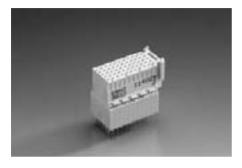
The ERmet type C vertical female connector provides 55 contacts in a 5 row x 11 position fully loaded configuration. Versions with optional "z" and "f" row shields are available as well as extended terminals for use in stacking applications with rear shrouds.
