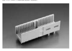
The ERmet male connector type M provides a maximum of 77 contacts in 7 rows by 11 positions. The two outer rows, z and f are for the shielding contacts of the male connector, along with 3 contact positions for special power or coax contacts. This type contains a multifunction cavity for coding and pre-alignment in the center position. This connector is designed to be used alone or in conjunction with either a type B, C, L, or N ERmet connector.
