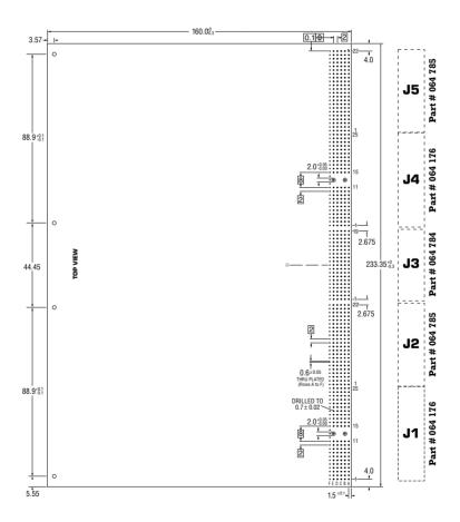
Note that the daughter card is numbered in accordance with the CompactPCI® specification. The numbering on the connectors themselves is different and in accordance with the IEC 61076-4-101 standard.
