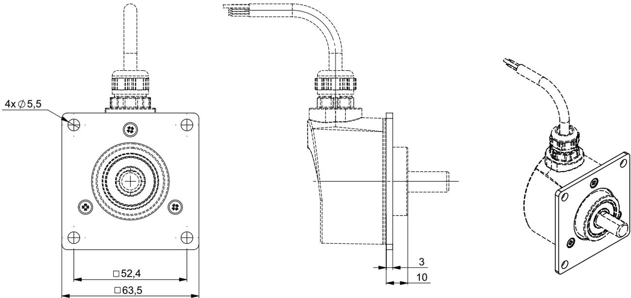
AH05\_14 Standard clamping, Connection BJR (Radial Cable), coupling 9445/012 mounted on the body
