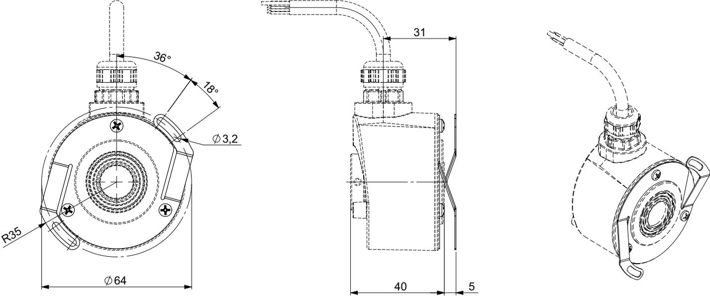
AH05\_14 Standard clamping, Connection BJR (Radial Cable), coupling 9445/015 mounted on the body
