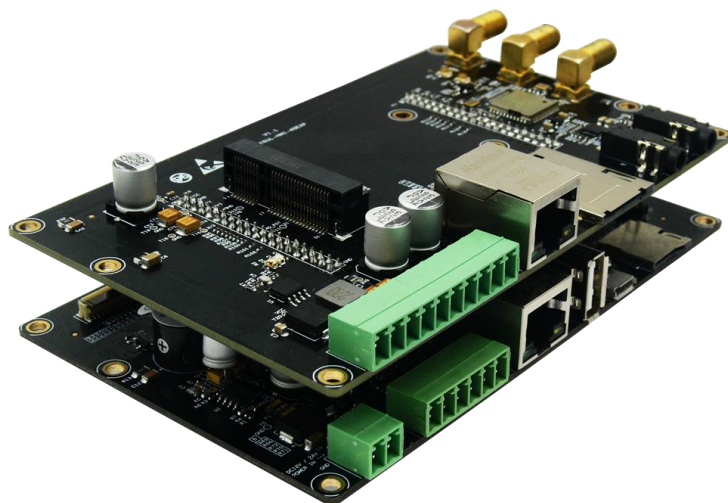
Figure 1-5 MYB-Y6ULX-HMI-4GEXP IO Board Mounted on MYD-Y6ULX-HMI Development Board
