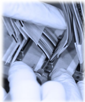
Potting a Micro-D with Epoxy-Filled Syringe
