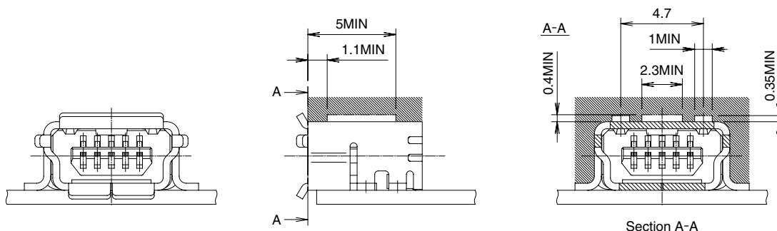
◆ Mated Assembly – Receptacle - with interface entry angle
