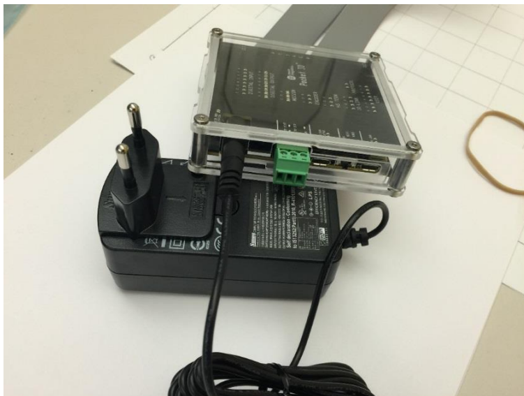
Figure 10. Pocket IO with Power Supply Connected.
